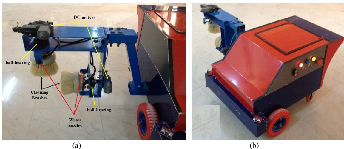
Fig. 1: The mobile robot (a) fixed cleaning arm (b) Robot body.
