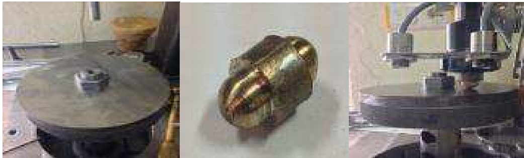
Fig. 1: Pin on disc machine and specimen
