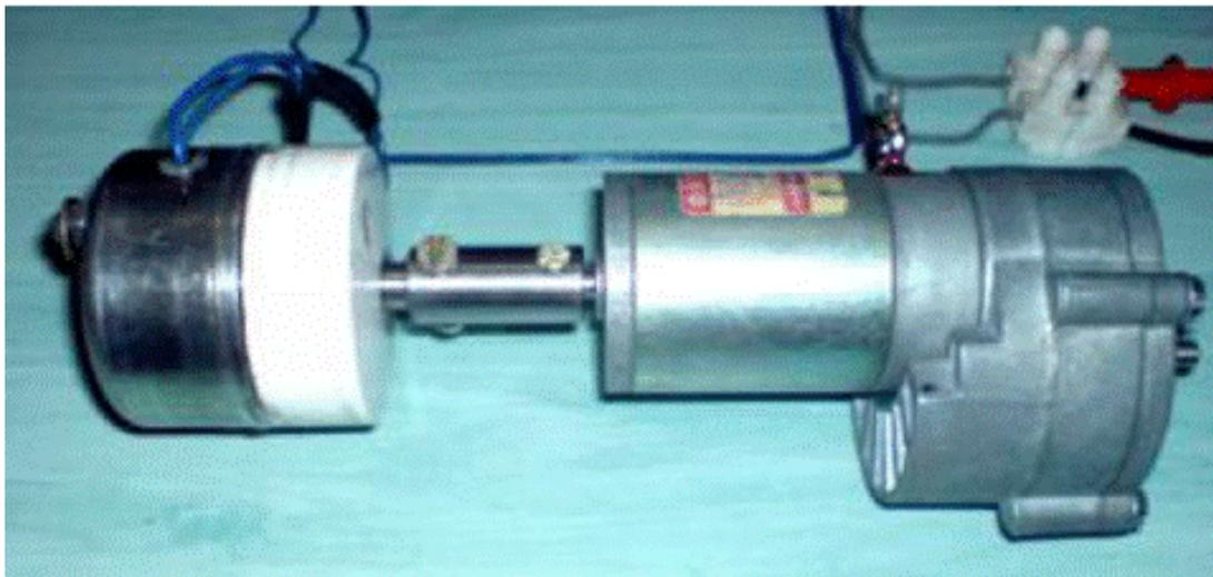
**Fig. 1:** Set up of coupling of brake and motor.
