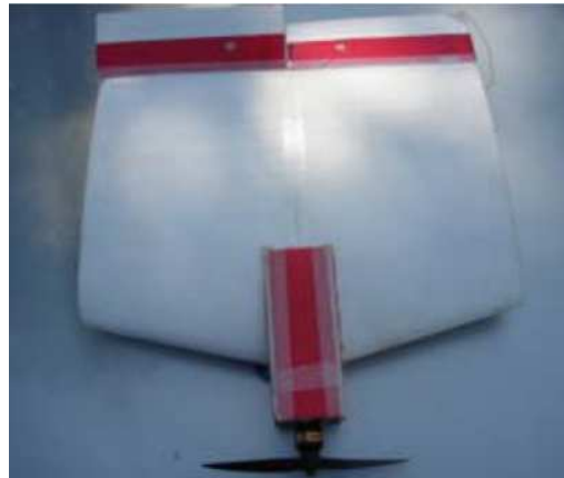
Fig. 5: MAV model without a vertical stabilizer(Tongchitpakdee, 2013)
