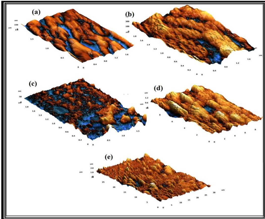
**Fig. 7:** AFM for the deposited  $\text{Bi}_{1.7}\text{Pb}_{0.3}\text{V}_x\text{Sr}_2\text{Ca}_2\text{Ti}_{0.3}\text{Cu}_{2.7}\text{O}_{10+\delta}$  films for different  $x$  [ (a) $x=0$ , (b)  $x=0.1$ , (c)  $x=0.2$ , (d)  $x=0.3$  and (e) $x=0.4$  after annealing process at  $800\text{ }^\circ\text{C}$
