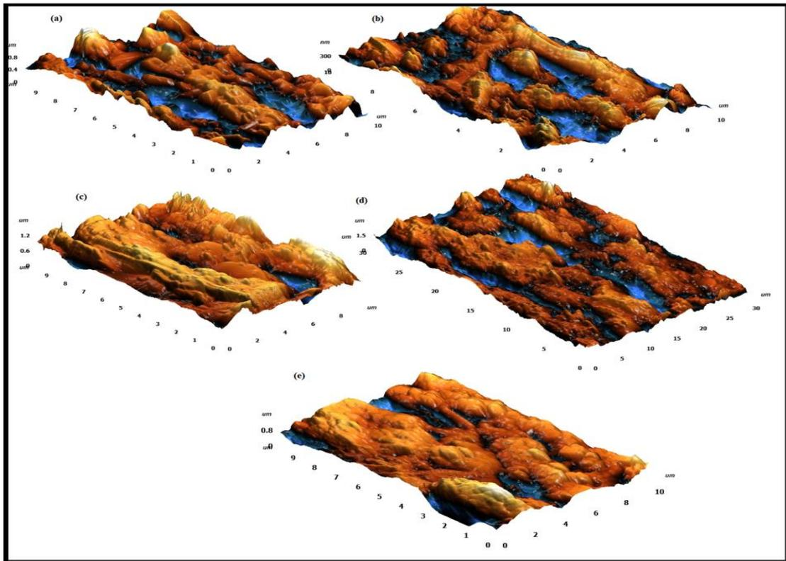
**Fig. 6:** AFM for the deposited  $\text{Bi}_{1.7}\text{Pb}_{0.3}\text{V}_x\text{Sr}_2\text{Ca}_2\text{Ti}_{0.3}\text{Cu}_{2.7}\text{O}_{10+6}$  films for different x [(a) x=0, (b) x=0.1, (c) x=0.2, (d) x=0.3 and (e)x=0.4] before annealing process at 800 °C.
