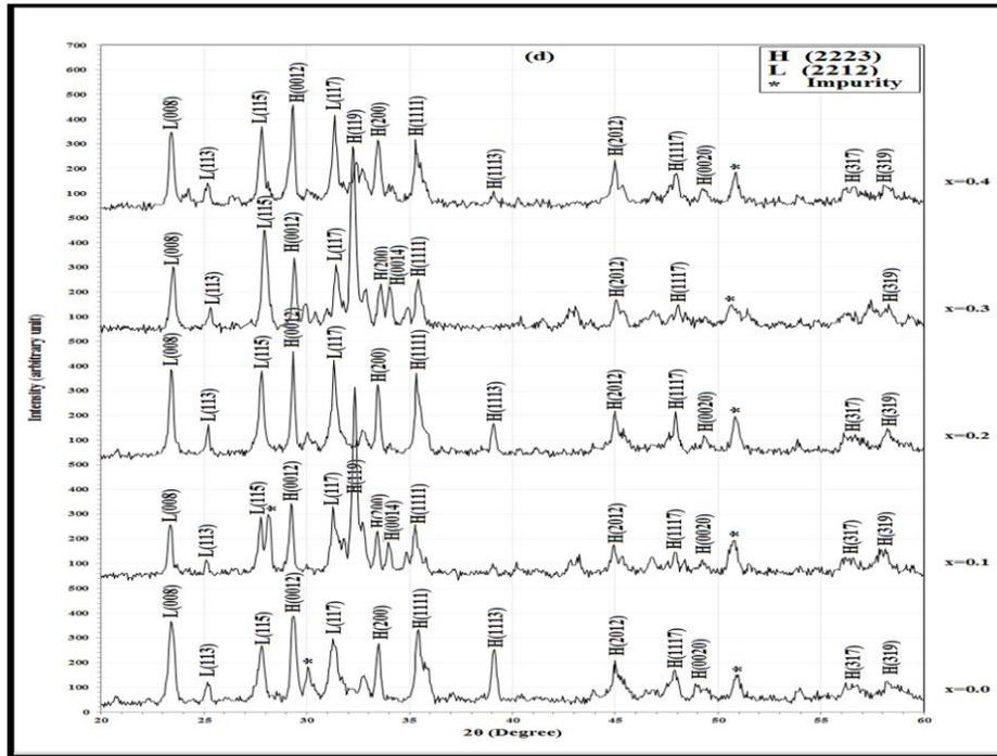
**Fig. 1:** XRD patterns for  $\text{Bi}_{1.7}\text{Pb}_{0.3}\text{Sr}_2\text{V}_x\text{Ca}_2\text{Cu}_{2.7}\text{Ti}_{0.3}\text{O}_{10+\delta}$  bulk samples for ( $x= 0.0, 0.1, 0.2, 0.3$  and  $0.4$ ) that sintered at  $835^\circ\text{C}$  for 140 h.
