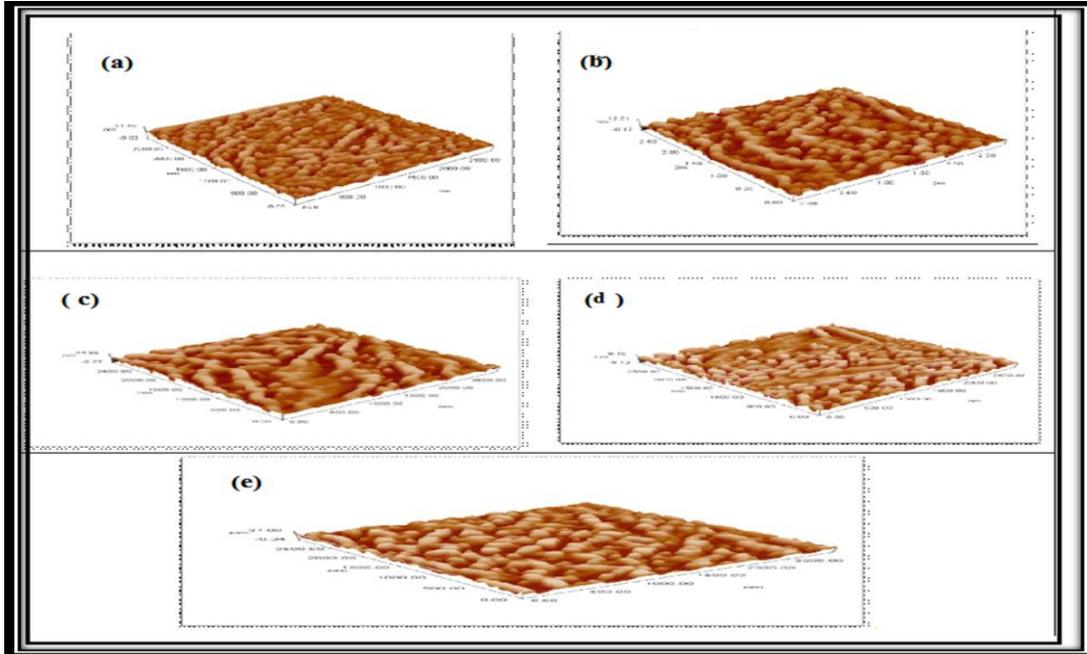
**Fig. 5:** AFM for  $\text{Bi}_{1.7}\text{Pb}_{0.3}\text{V}_x\text{Sr}_2\text{Ca}_2\text{Ti}_{0.3}\text{Cu}_{2.7}\text{O}_{10+6}$  bulk samples for different x (a)x=0, (b) x=0.1, (c) x=0.2, (d) x=0.3 and (e)x=0.4.
