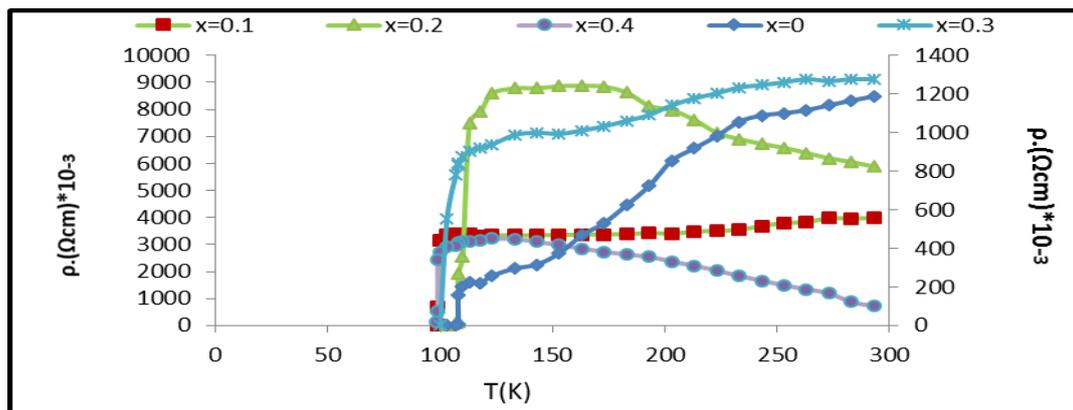
**Fig. 4:** Temperature dependence of resistivity for the deposited  $\text{Bi}_{1.7}\text{Pb}_{0.3}\text{V}_x\text{Sr}_2\text{Ca}_2\text{Cu}_{2.7}\text{Ti}_{0.3}\text{O}_{10\pm\delta}$  films on Si substrate for different x (0,0.1, 0.2,0.3and 0.4).
