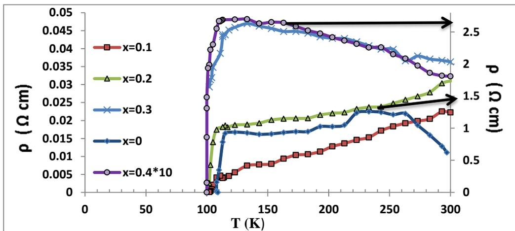
**Fig. 3:** Temperature dependence of resistivity for  $\text{Bi}_{1.7}\text{Pb}_{0.3}\text{V}_x\text{Sr}_2\text{Ca}_2\text{Cu}_{2.7}\text{Ti}_{0.3}\text{O}_{10+\delta}$  system for different V concentration that sintered at  $835^\circ\text{C}$  for 140h.
