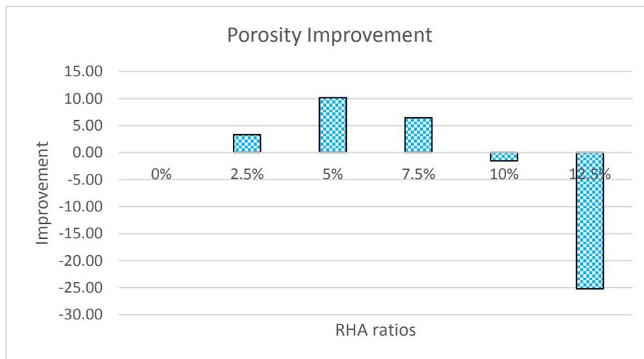
Figure 8: Evolution of porosity improvement as a function of rice husk ash mass fraction
