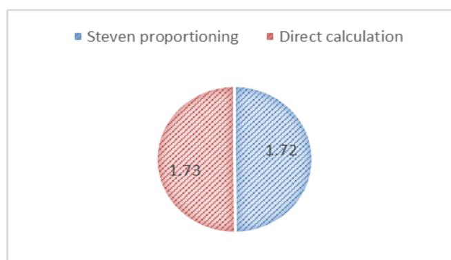
Figure 6: Mass of CO<sub>2</sub> released during the complete combustion of 1Kg of rice husk
