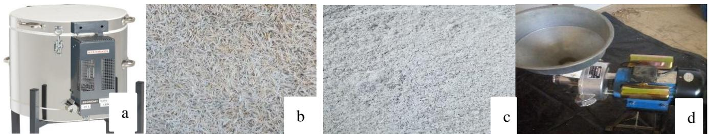
Figure 2: kiln (a), unground RHA (b), ground RHA (c), grinder (d)
