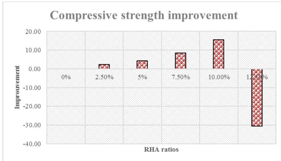
**Figure 9:** evolution of compressive strength improvement as a function of rice husk ash mass fraction
