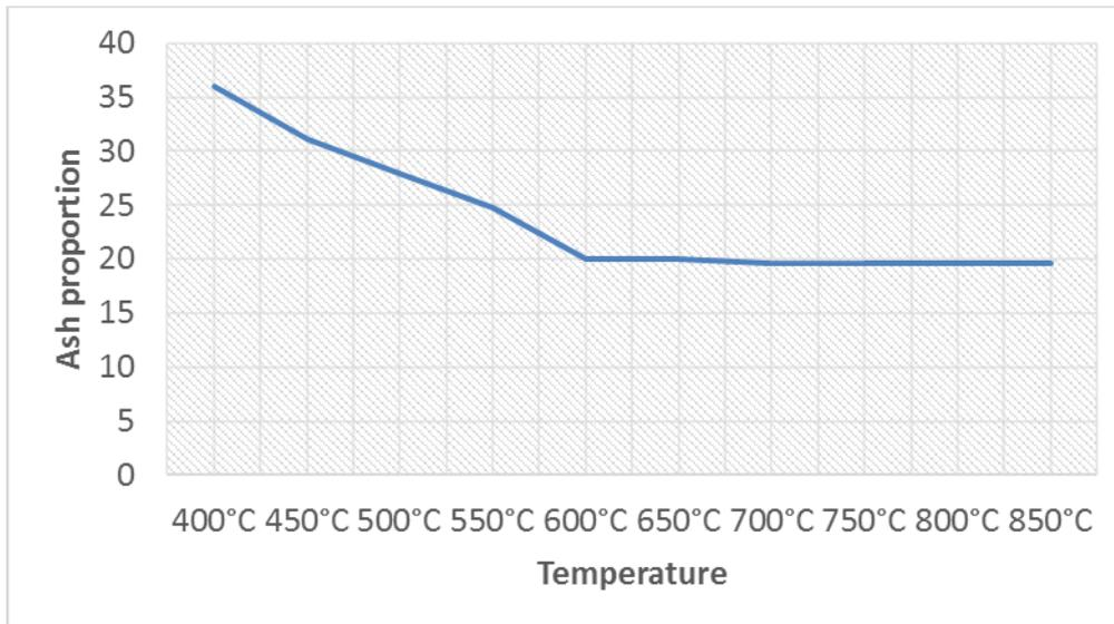
Figure 5: Evolution of the rice husk ash mass as a function of calcination temperature
