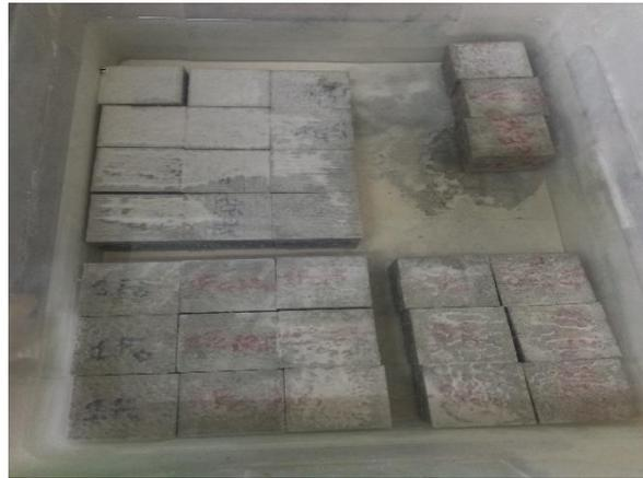
**Figure 3:** Specimen curing condition
